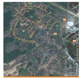
Example of grid mapping Red line: main grid Orange lines: secondary grid Blue lines: tertiary grid
